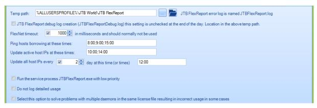
**Temp path** – A temporary path where the HTML reports are created and some other temporary files are created. Use this if you have problems with the rights on the HTML file when users try to access it. If specified the debug log and error log will be placed in this folder.
