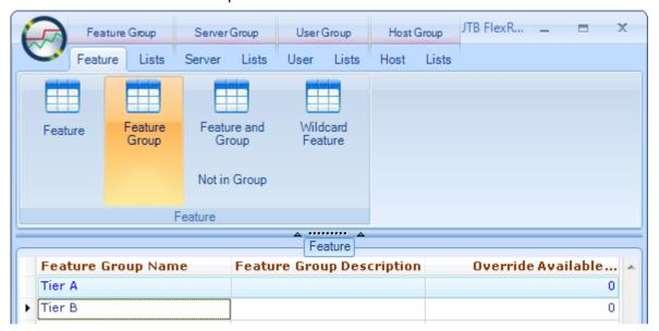
Feature and Group is used to connect a feature name with a feature group one by one.
