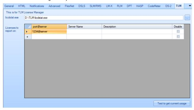
**licdstat.exe:** TLM is running on another computer it is recommended to take a copy of licdstat.exe and place it on the same computer as JTB FlexReport Core is installed.
