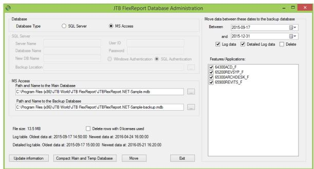
When working on the main backend database stop the JTB FlexReport Core Service in JTB FlexReport Config and start it when ready. It is recommended to stop all other JTB services during this time as well. After deleting or moving data it is recommended to run JTB FlexReport Service Configurator and click on Clear followed by Sampling All Records in the Sampling to Cache area.
