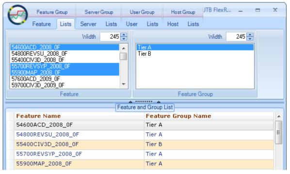
To **delete** or disassociate/disconnect multiple rows at a time use any of the List tabs. Select in the grid and press Delete.
