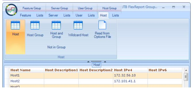
This show the usage of Wildcard Hosts. Click on the Wildcard Host button. Use the dropdown in the Item Type column to select either Host, HostIPv4 or HostIPv6. Press Enter for a new row.
