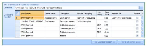
**Lmutil.exe** - Lmutil is the path and file name for lmutil.exe. This is a required and should normally be the installation location of JTB FlexReport Core.
